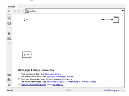
The new untitled model, with the default solver set to VariableStepAuto, contains a Solver Configuration block, a Simulink-PS Converter block, and a PS-Simulink Converter block connected to a Scope block.
