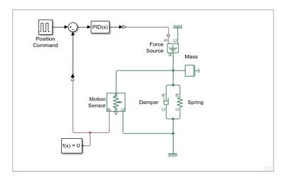
The control Simulink signal goes to the input port of the Simulink-PS Converter block, where it is converted into a physical signal driving the force profile of the Ideal Force Source block.
